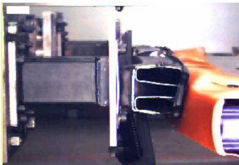
Figure 9: Cross over Vehicle Bumper System Showing Beam Buckle in Physical Test
